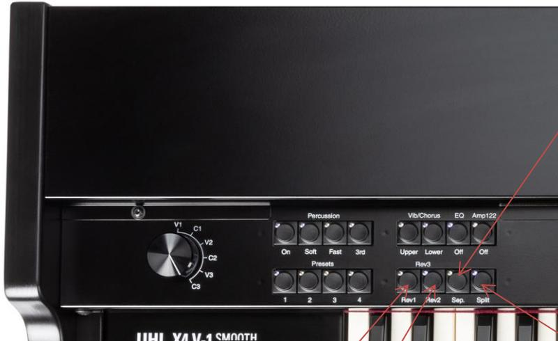
**Sep.** (Separate bass): The pedal bass is always separately available at the "Separate Bass" output socket on the back of the organ. With the "Sep." button you can switch off the pedal bass at the outputs "Main-Out L + R", "Pure Organ" and "11-Pin". The pedal bass is now connected to the mixer via the "Separate Bass" output. Now you can mix the Pedalbass completely detached from the rest of the organ (volume, possibly EQ).
