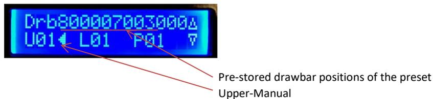
Now set the real drawbars of the Upper-Manual as desired. The changes in the drawbars are shown in the display behind Drb (Drawbar):
