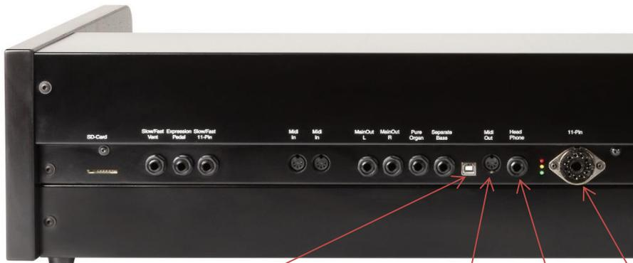
**USB:** The USB socket of the UHL X4 V is sealed - it is used exclusively for service work on the part of the manufacturer. Removing the USB cap can void the manufacturer's warranty.
